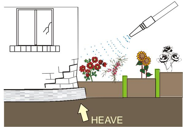
Fig. 9 Slab heave due to water ponding
