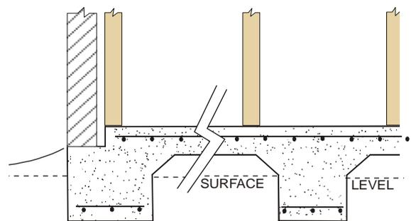
Fig 2 Waffle Slab
