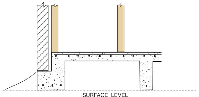
Fig. 3 Strip & Stump Footing System
